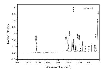
Figure 7: FT-Raman Spectrum of La<sup>3+</sup> doped mNA single crystal
