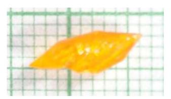
Figure 2: Photograp of La<sup>3+</sup> doped mNA crystal
