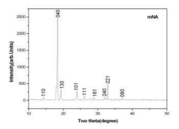
Figure 3: XRD pattern of pure mNA single crystal
