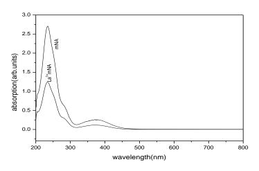
Figure 5: UV-Vis Spectrum of pure and La<sup>3+</sup> doped mNA single crystal
