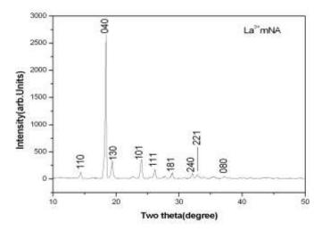
Figure 4: XRD pattern of La<sup>3+</sup> doped mNA single crystal
